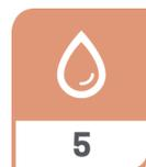
**Fluid Resistance:** This is a subjective attribute rating of "1 - 5". 1 being the least fluid resistant and 5 being the most fluid resistant. This is based on actual test data in accordance to ISO 6722-1, SAE, or UL. Insulation materials are not uniformly resistant to all chemicals. Specific chemical resistance is found on the back of the data sheets.
