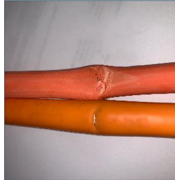
Cables after pinch force test. Top: EXTRAD thin -wall. Insulation intact (95lbs) Bottom: Rubber thick -wall. Insulation severed (80lbs)
