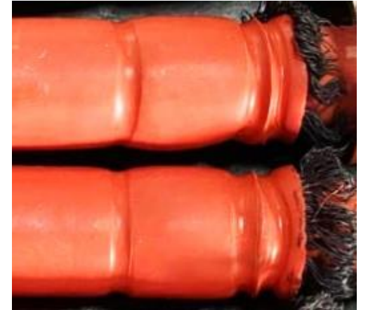
Deformation caused by connector pressure at elevated temperatures
