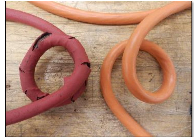
3000hr 150°C Heat Aging: Left: 150°C chemically crosslinked XLPO Right: 150°C Irradiated EXTRAD ERGO-FLEX XLPO
