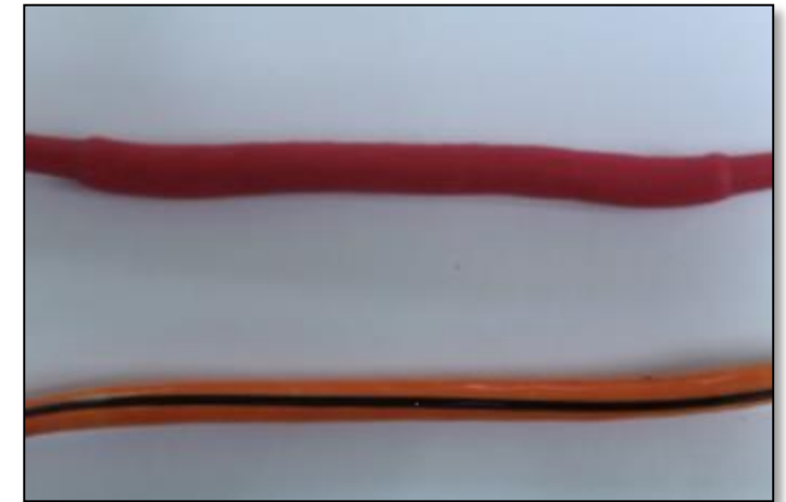
ISO-6722-1 Oil Swell. Max allowable = 15% Top: Chemically crosslinked EPDM. 95% Swell. Bottom: Irradiated EXTRAD XLPO. 9% swell.
